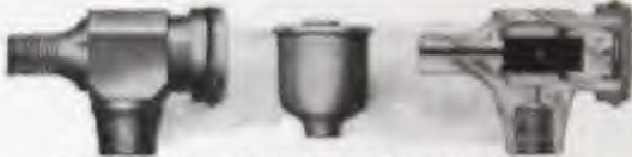
No. B 3344. AUTOMATIC AIR VALVE For Steam Radiators and Coils. Nickel plated. Screwed 1 in. Gas. Before fitting, loosen screw (B), then fit the valve, and when the radiator becomes too tight, the screw gradually until there is no escape of steam at outlet (D). Then screw on the cap tightly to prevent interference with the adjustment. Drop cap to screw at outlet, extra. Extra composition plug can be supplied.
